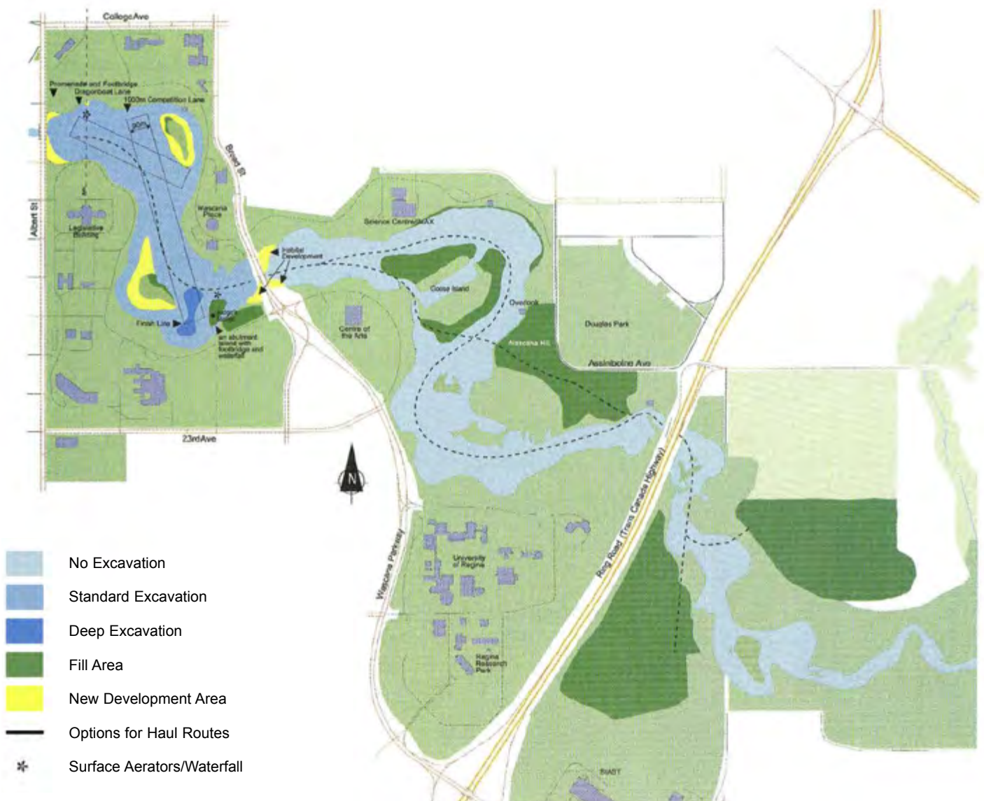
2003-2004 Big Dig Plan with areas of excavation (in blue) and areas of fill (in dark green). There were a few changes to this plan: the fill around Goose Island did not occur, and a new island was created between the Science Centre and the Display Ponds.
